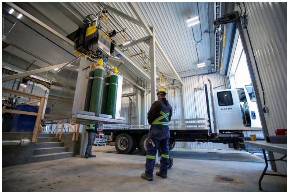
Figure A-40 The transport pod is loaded onto a truck to take fish upstream of the dam site to be released back into the Peace River and its tributaries (October 2020)
