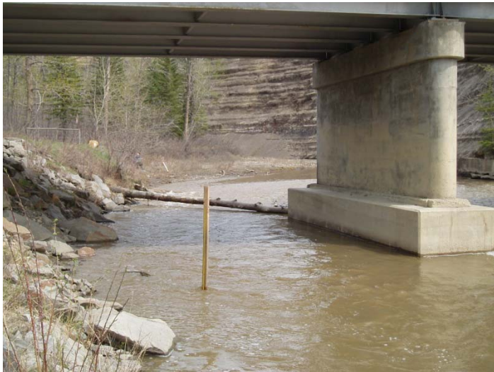
Photograph 14: The staff gauge affixed to an old wooden piling in Farrell Creek. Cache Creek and Lynx Creek required measurements to the water level from a bench mark.
