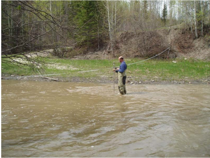
Photograph 13: Taking a discharge measurement at Lynx Creek during May 2007.
