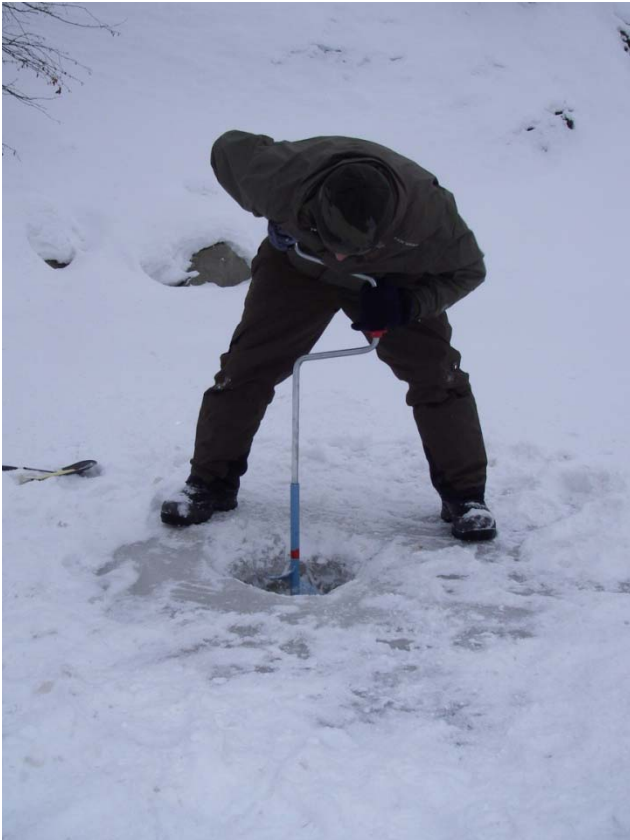
Photograph 10: Ice augers used in March 2007 to access water for sampling in tributaries.
