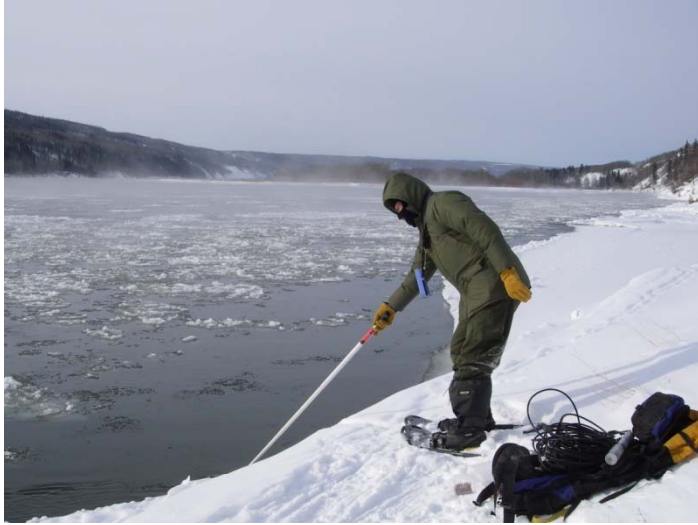
Photograph 9: Water samples collected from the Peace River during the winter were completed from shore using an extendable pole with a sampling vessel attached to the end of the pole as shown here in March 2007.
