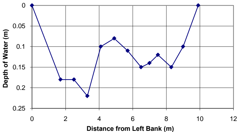
Flow Measurement Section at Lynx Creek
