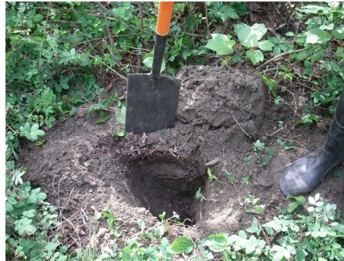
Photograph 5: Soil pit sampled at the Halfway River at Site 25, 1.5 km upstream of the confluence with the Peace River. Sands comprised most of the soil at this site.
