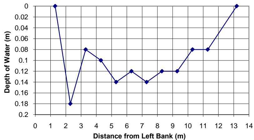
Flow Measurement Section at Cache Creek
