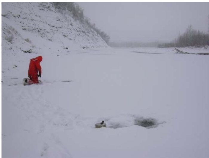
Photograph 1: Installing temperature data loggers on the Kiskatinaw River in November 2006. Although prior to the onset of a major winter storm, access was still difficult due to developing ice and snow.
