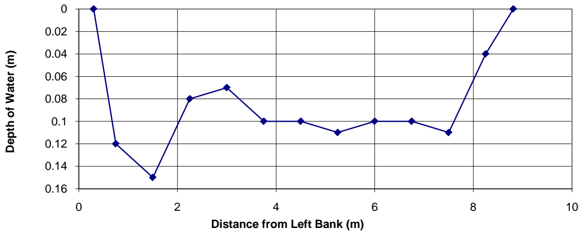
Flow Measurement Section at Lynx Creek
