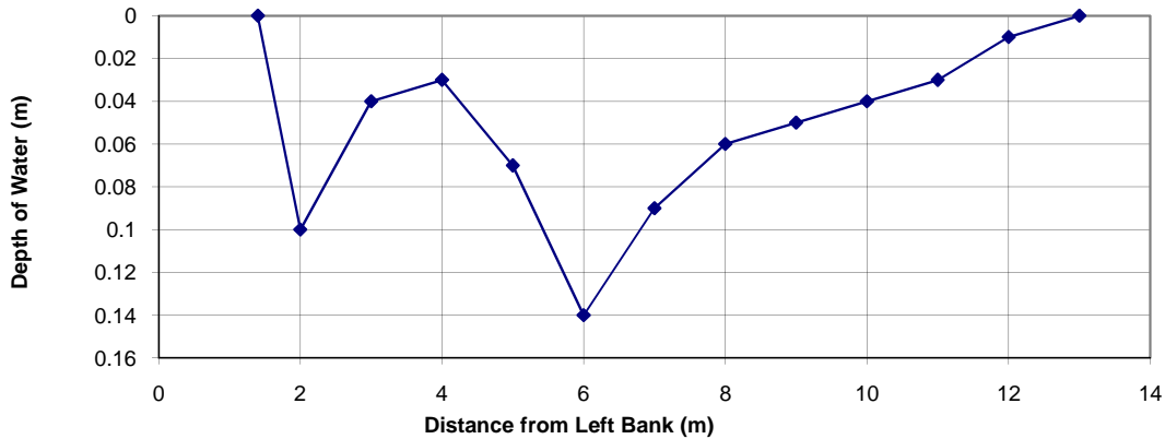
Flow Measurement Section at Cache Creek
