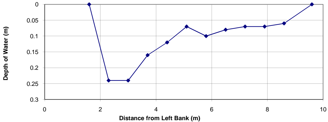
Flow Measurement Section at Cache Creek
