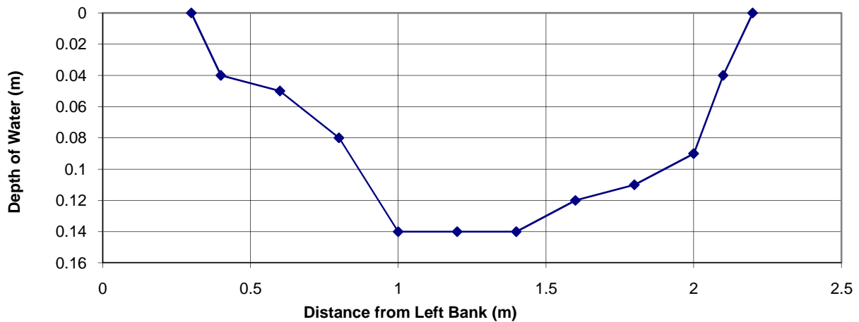
Flow Measurement Section at Boudreau Creek
