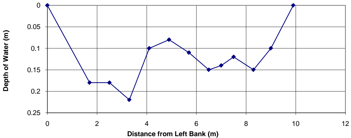
Flow Measurement Section at Lynx Creek
