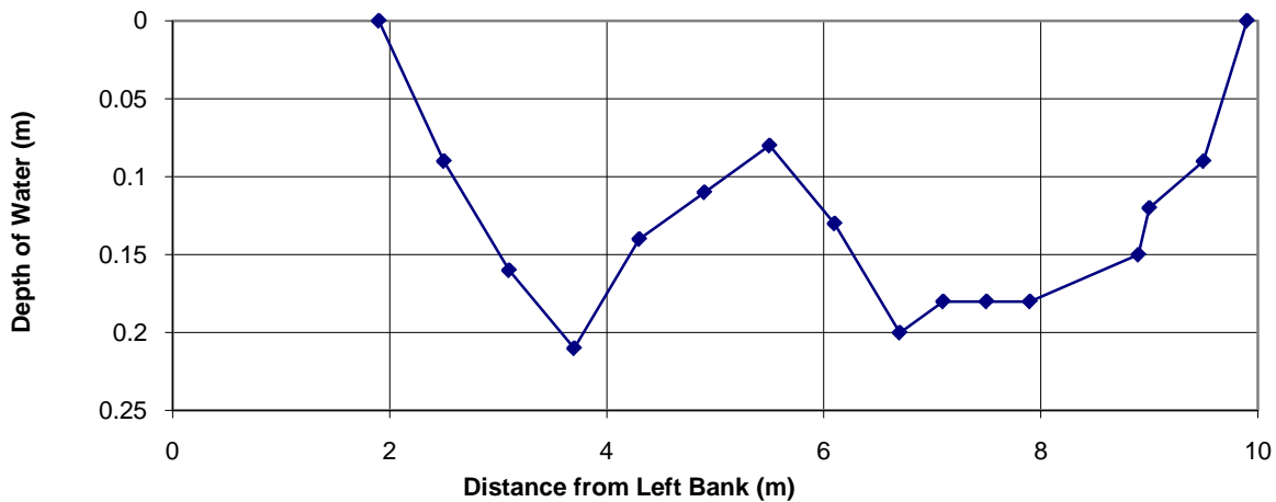
Flow Measurement Section at Lynx Creek
