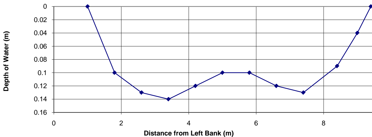
Flow Measurement Section at Lynx Creek
