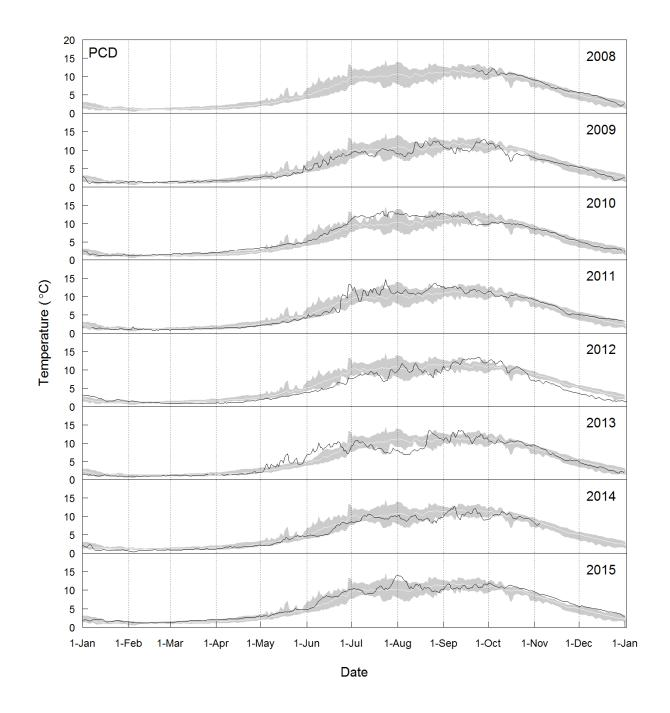
Figure C3: Mean daily water temperature (°C) for the Peace River at Peace Canyon Dam (PCD; black line), 2008 to 2015. The shaded area represents minimum and maximum water temperatures recorded at PCD during other study years between 2008 and 2015. The white line represents average mean daily water temperatures over the same time period. Data were collected under GMSWORKS-2 (DES 2014).
