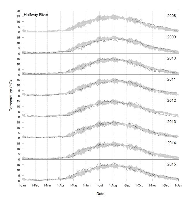
Figure C4: Mean daily water temperature (°C) for the Peace River downstream of the Halfway River confluence (black line), 2008 to 2015. The shaded area represents minimum and maximum water temperatures recorded at the site during other study years between 2008 and 2015. The white line represents average mean daily water temperatures over the same time period. Data were collected under GMSWORKS-2 (DES 2014).
