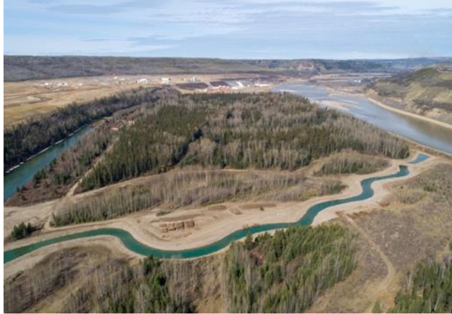
Figure A-9 Newly built side channels on the Peace River provide fish habitat (June 2019).
