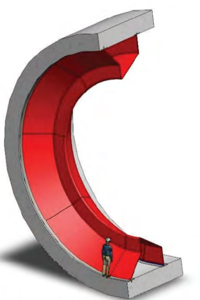
Cross Section of Diversion Tunnel 2 - orifice
