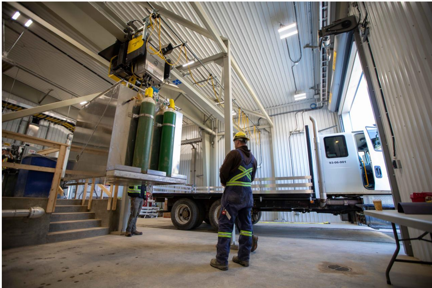
Photo 8. Workers load a transport pod onto the transport truck using the monorail crane hoist inside the sorting facility (October 2, 2020).
