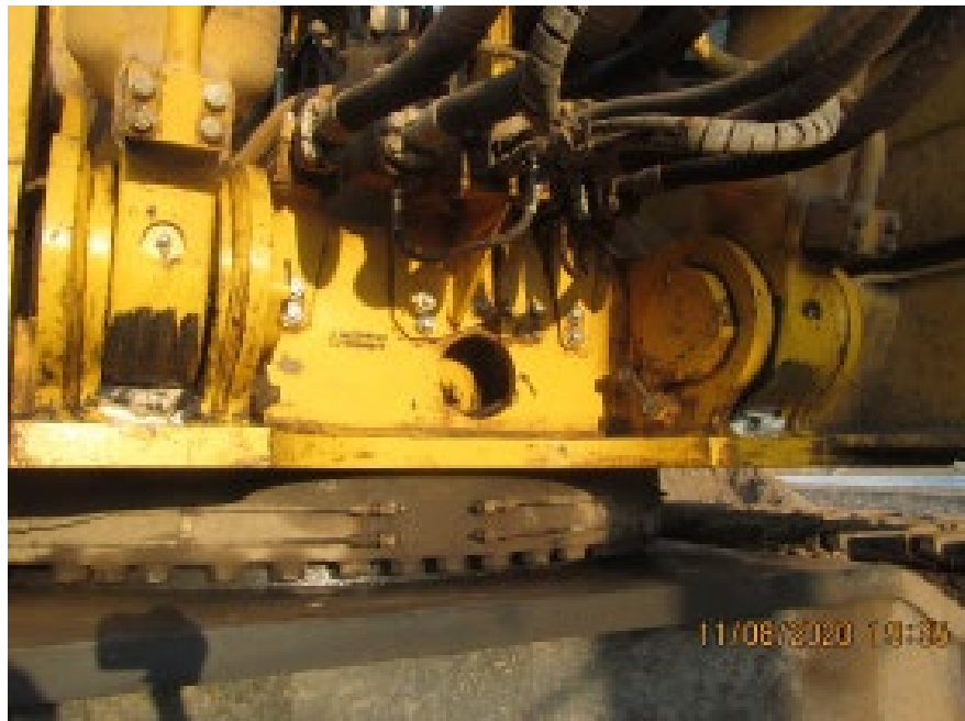
Figure 2. Within the dam site construction area all in-river machines are regularly checked for any signs of over greasing (August 11, 2020).
