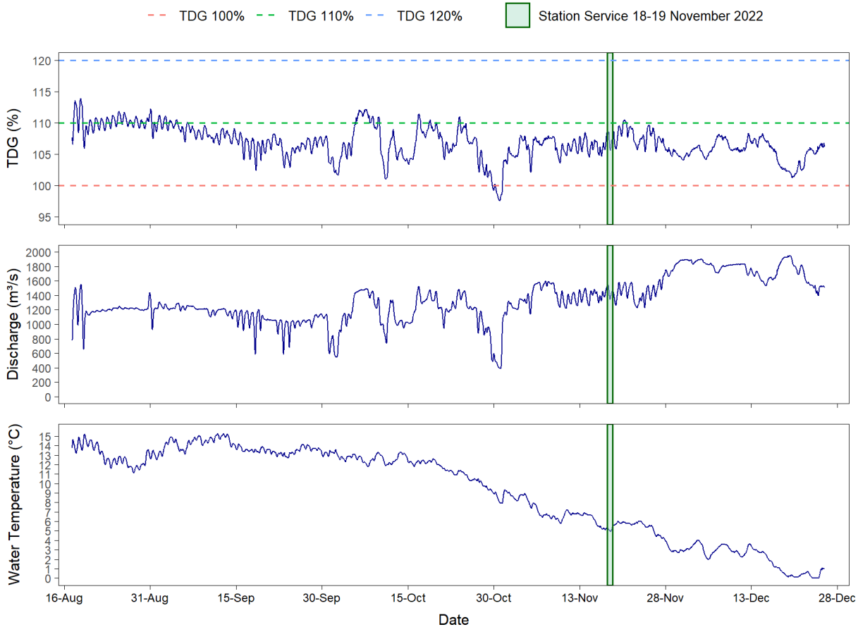
Figure 4: A hourly time-series comparison of percent TDG and water temperature recorded at Stn_112.5L in relation to Peace River total discharge, 17 August to 27 December 2022. The dash lines in the top panel correspond with BC Hydro TDG guidelines in British Columbia (BC Hydro 2014, 2022) in relation to the risk for gas bubble trauma in fish. The green vertical bar indicates the timing of the service visit to the station.
