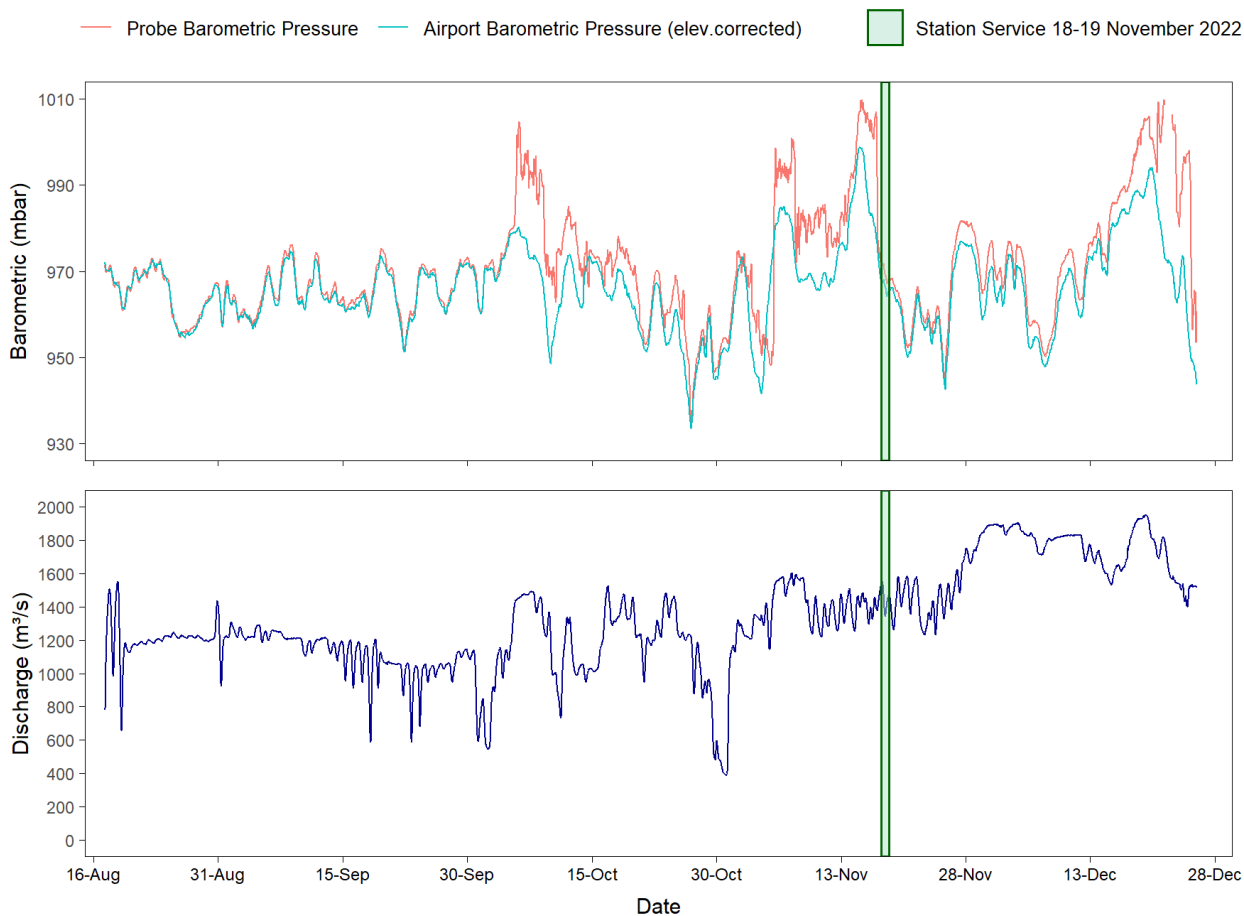
Figure 8: Barometric pressure measured by the TDG station in relation to calculated barometric pressure at the station and total river discharge (Station 07FA004) from 17 August to 12 December 2022. Green vertical bar indicated the dates that service visits were conducted at the station.
