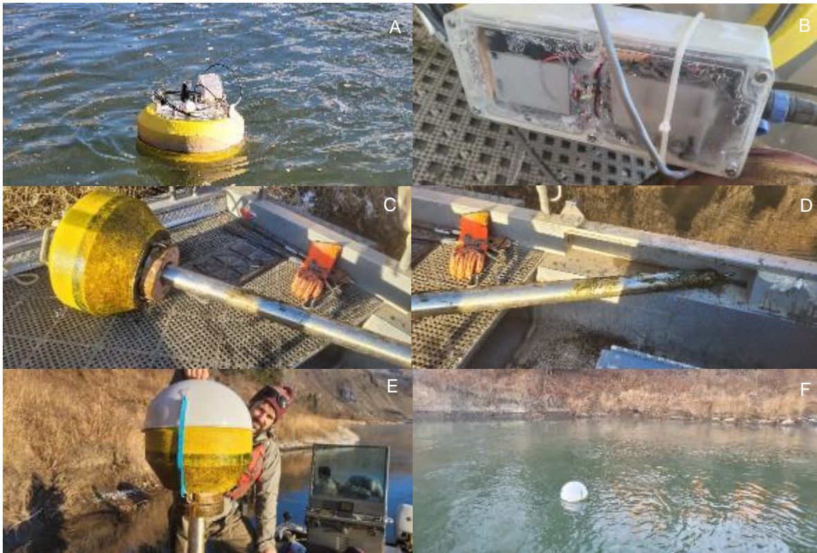
Figure 9: TDG station at Stn_112.5L without its fabric cover (A), water-damaged power supply (B), biofouling of station buoy, instrument tube, and TDG probe (C and D), new acrylic dome cover (E), and the deployed station after servicing (F).
