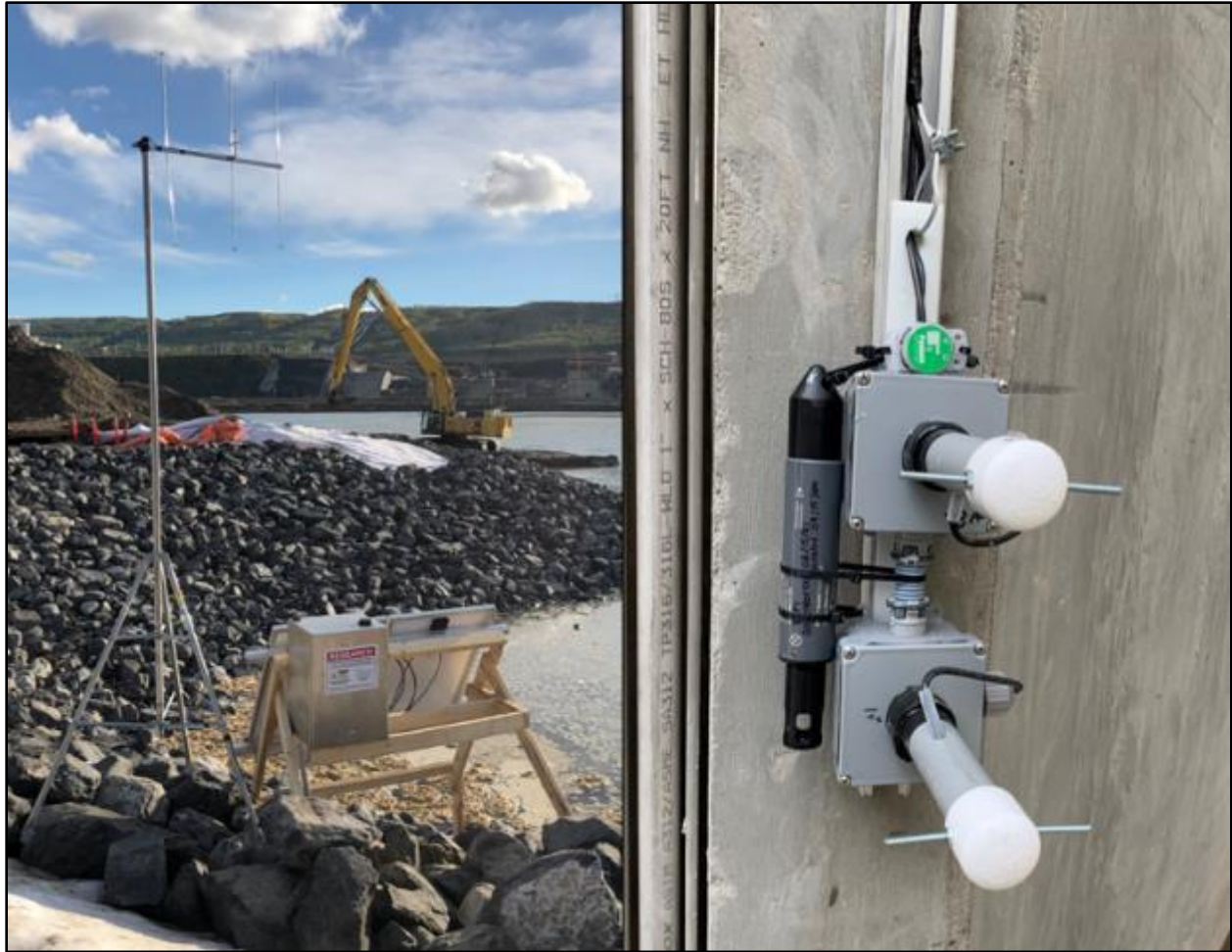
Figure 6. An aerial antenna (left) and two dipole antennas (right) at fixed stations within the Mon-13 study area. A dissolved oxygen logger and a light and temperature logger are also affixed to the dipole housing (right).
