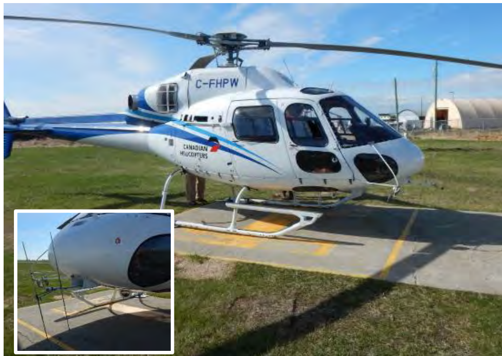
Figure 7. Twin-engine helicopter equipped with a single H-antenna mounted on the nose for conducting mobile-tracking surveys.
