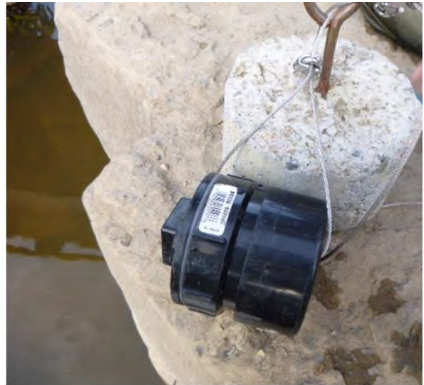
Figure 2: Examples of temperature logger housings deployed during the Site C Reservoir and Peace River Water Temperature Monitoring Program (Task 2b). The photo on the left denotes housings initially deployed during GMSWORKS-2. The photo on the right denotes housings initially deployed during Task 2b.
