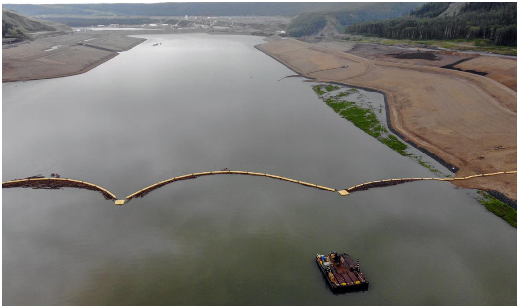
Figure A-14 An aerial view of the headpond and debris boom where a barge is used for clearing debris materials from the boom (July 2021)
