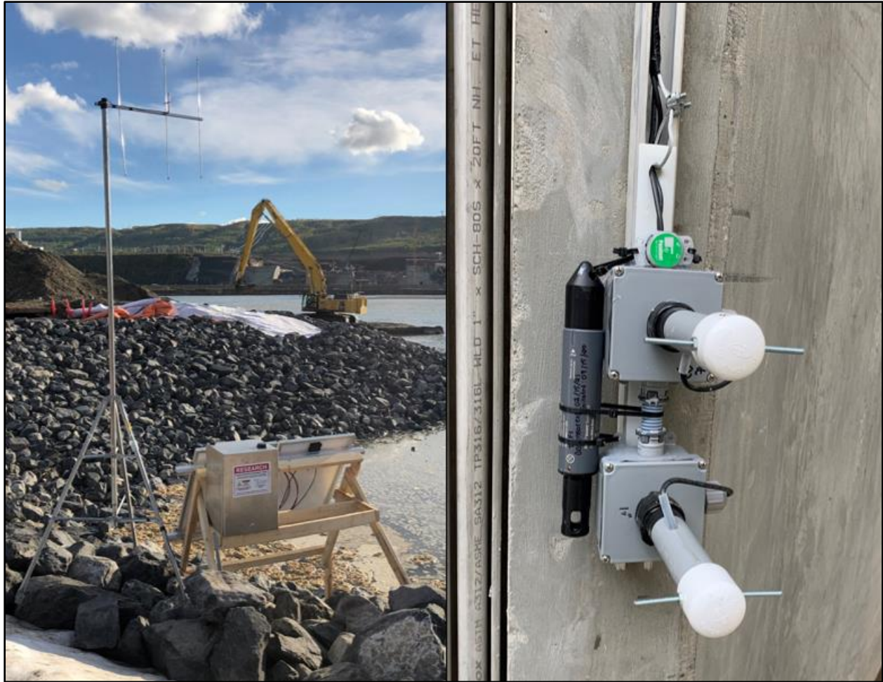
Figure 7 An aerial antenna (left) and two dipole antennas (right) at fixed stations within the Mon-13 study area. A dissolved oxygen logger and a light and temperature logger are also affixed to the dipole housing (right).
