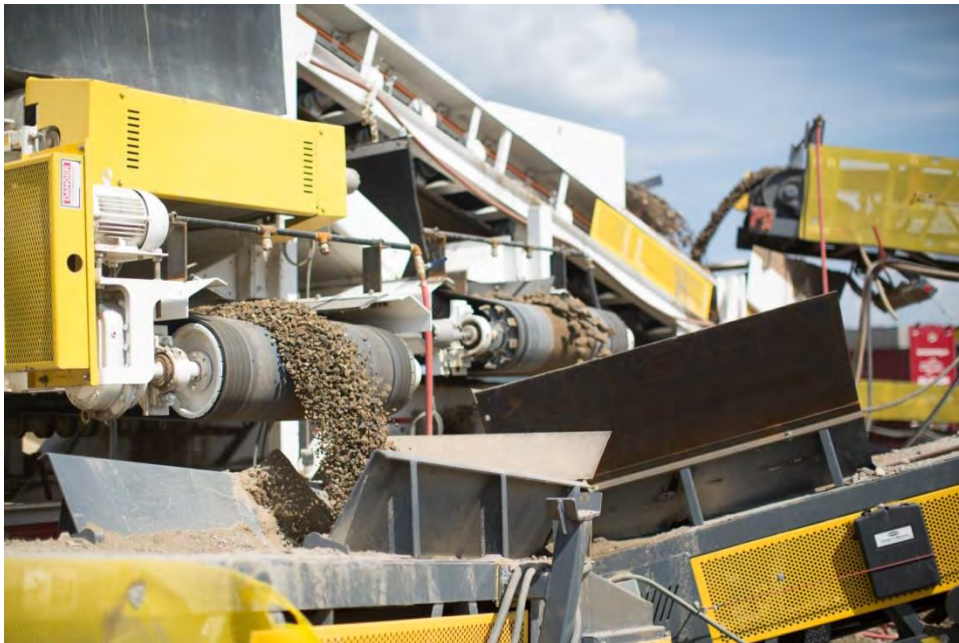
Figure A-20 Aggregated Crushing Equipment on the South Bank (June 2017)
