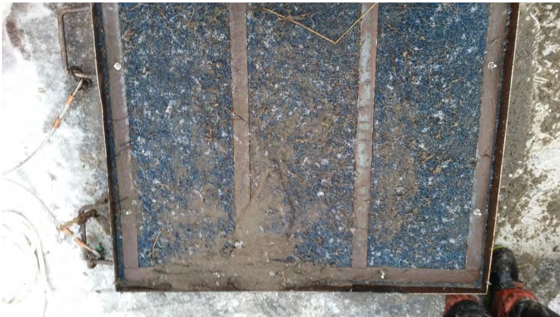
Plate 3 Sand and fines deposited onto substrate mat M09 on 4 January 2019.
