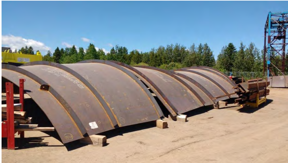
Figure A-7 Manufacturing of Units 1 to 6 Draft Tube Elbows and Cones in Progress at LAR Machinerie, Quebec. Photo taken June 13, 2017.
